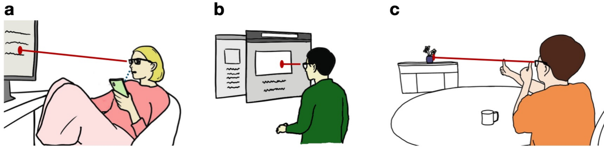
Fig. 2. Applications of VergeIO. (a) Varifocal lenses adjust focal depth as the user shifts gaze between ambient reference points: a nearby phone and a distant TV. (b) Smart glasses enable gaze-based selection between virtual objects at different depths. (c) Remote screening of ocular disorders using approximate reference points: thumbs and a distant object.
